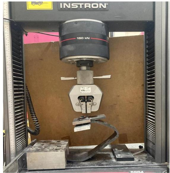
Figure 4. Visuals of sample fixed for quasi-static bending test.
