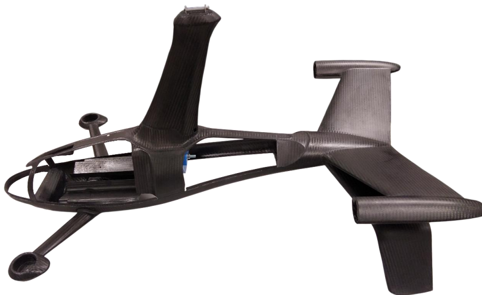
Fig. 2. View of the first version of the UAV fuselage as prepared for strength tests.
