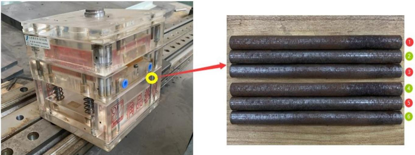
Fig. 4. Schematic diagram of six specimens from the mold.
