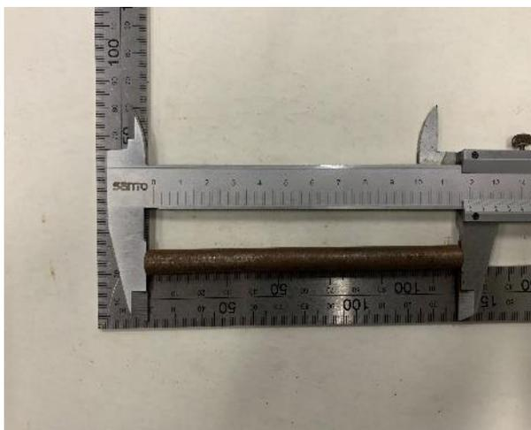
Fig.5. Length measurement of the pin part.
