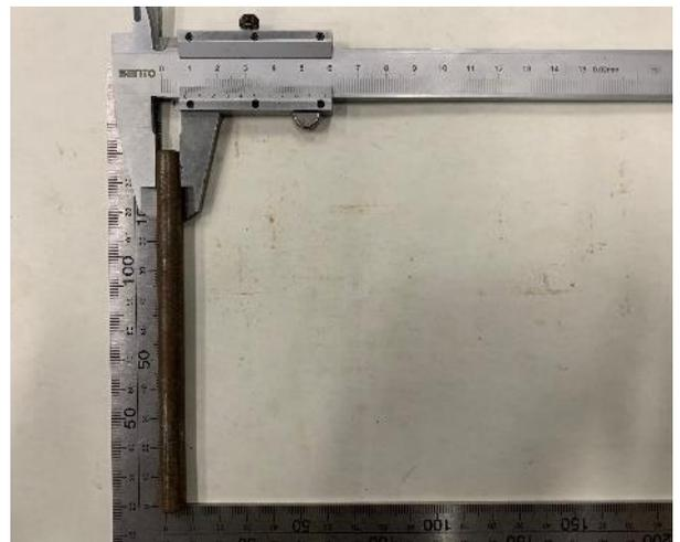
Fig. 6. Diameter measurement of the pin part.
