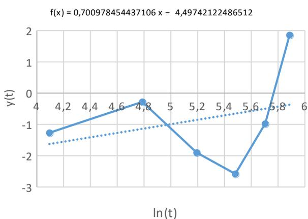
Figure 9. Calculated  $y(t)$  values as a function of  $\ln(t)$  by using measured Sa values for anode plate.
