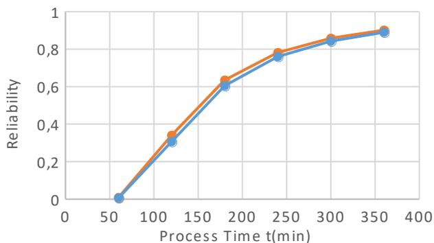
Figure 11. Calculated reliability roughness (RMS) and mean roughness (Sa) for Al surface placed at cathode.
