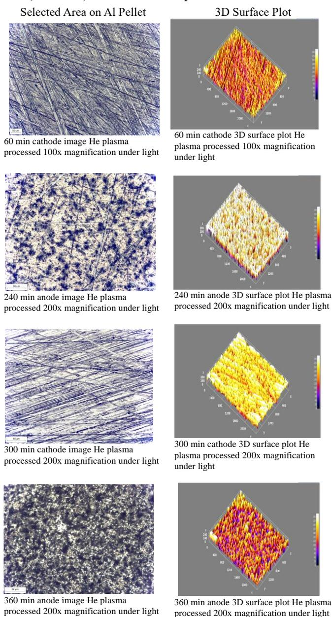
Figure 3. Al surface observation images and their 3D plot graph of anode and cathode with different process time of He plasma on Metal Microscope.
