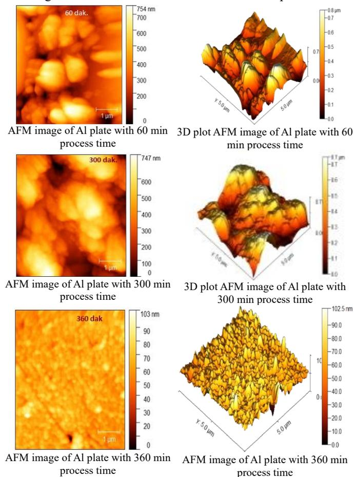
Figure 5. AFM images and 2D and 3D profiles of Al plates under 0, 300 and 360 min process time.
