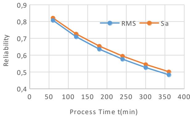
Figure 10. Calculated reliability roughness (RMS) and mean roughness (Sa) for Al surface placed at anode.
