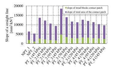
Fig. 17. The measure of the intensity of the changes in the area of contact between the wheels and the rigid ground, caused by an increase in the normal load (in the case of PTs, with each inflation pressure highlighted).
