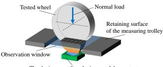
The device recording the image of the contact patch between the wheel and the road
