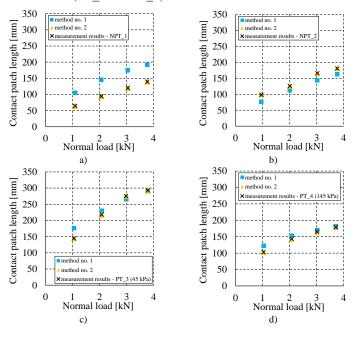
Fig. 16. Comparison of the measured and calculated contact patch lengths of selected wheels: a) NPT\_1, b) NPT\_2, c) PT 3 (45 kPa), d) PT 4 (145 kPa).
