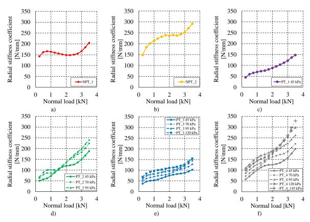
Fig. 11. Changes of radial stiffness coefficient as a function of normal load: a) NPT 1, b) NPT 2, c) PT 1, d) PT 2, e) PT 3, f) PT 4.
