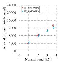
Fig. 13. Exemplary results of contact patch's area measurement as a function of normal load in two sections of the PT\_4 (70 kPa).
