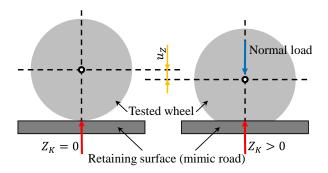
Fig. 3. Principle of measurement of radial stiffness characteristics.
