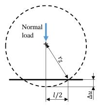
Fig. 6. Tire deformation and contact patch length due to normal load (figure based on [25]).
