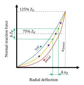
Fig. 4. Methodology for determining the radial stiffness coefficients for the i-th range of normal load.
