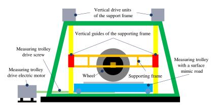
Fig. 1. Universal Test Bench for Quasi-Static Tire Research.
