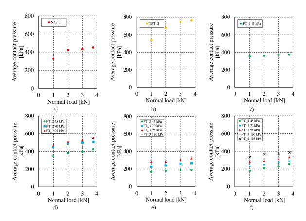
Fig. 15. Change of the contact pressure value in the contact patch of the tread blocks with the non-deformable ground as a function of normal load: a) NPT 1, b) NPT 2, c) PT 1, d) PT 2, e) PT 3, f) PT 4.
