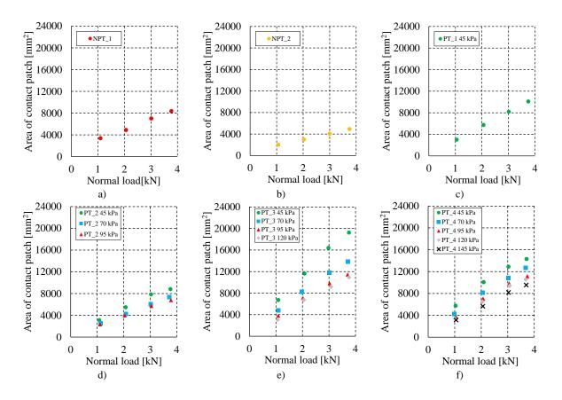
Fig. 14. Change of the area contact patch as a function of normal load: a) NPT 1, b) NPT 2, c) PT 1, d) PT 2, e) PT 3, f) PT 4.
