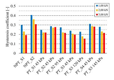
Fig. 8. Calculated values of the hysteresis coefficient of the research objects.
