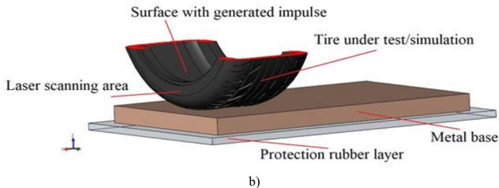
Fig. 4. The experimental details (the graphs from the measuring): a) test bench for measuring; b) scheme of measurement setup.
