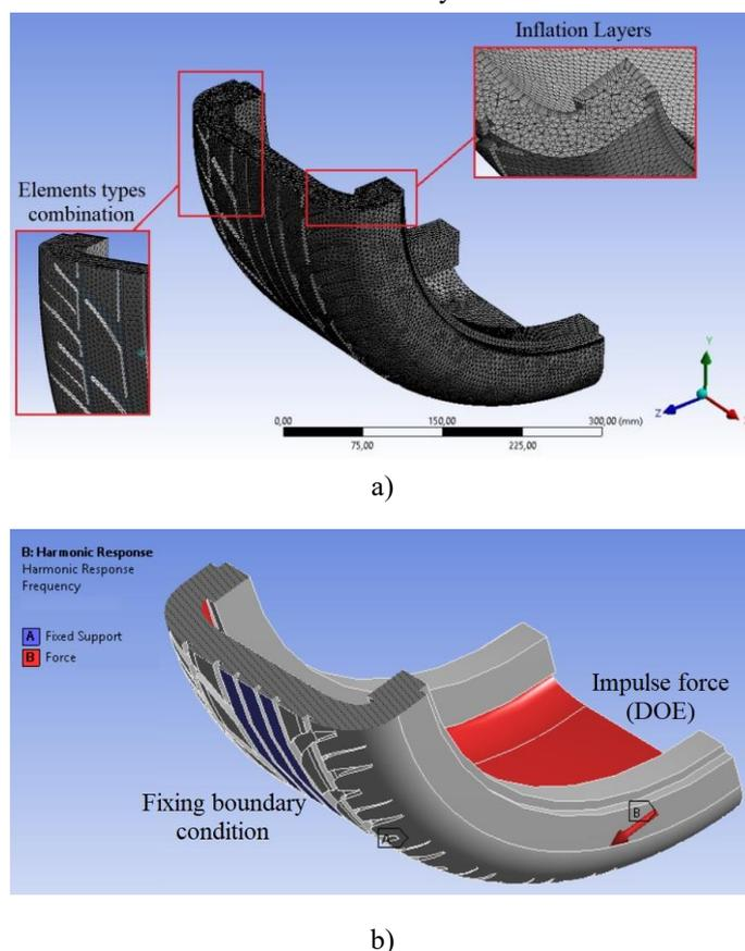
Fig. 2. View of numerical model parameters: a) example of grids in mesh independence study; b) view of the boundary conditions for numerical modelling.
