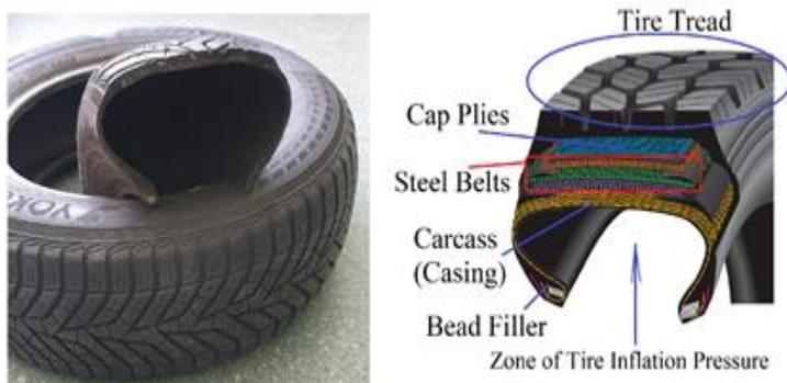
Fig. 1. Composite pneumatic tire construction (based on [6]).
