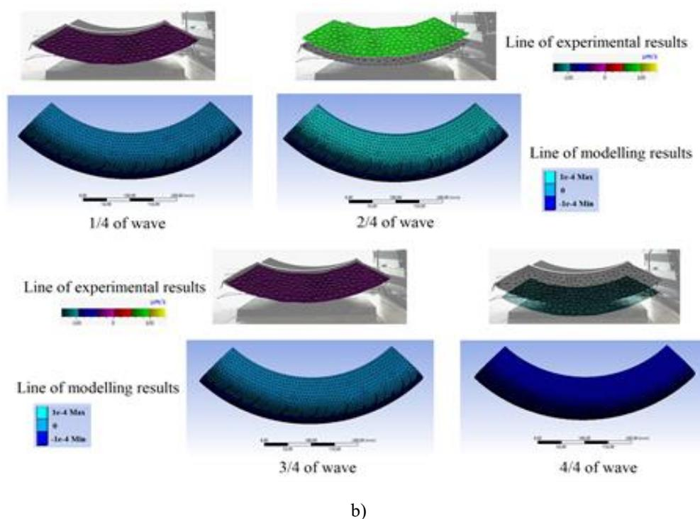
Fig. 8. Front surface deformation of composite tire material from experimental and numerical results: a) deformation on first resonance frequency (20 Hz); b) velocity of deformation on frequency of generated impulse (50 Hz).
