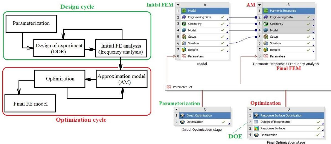
Fig. 3. Flowchart of the optimization task in ANSYS software.
