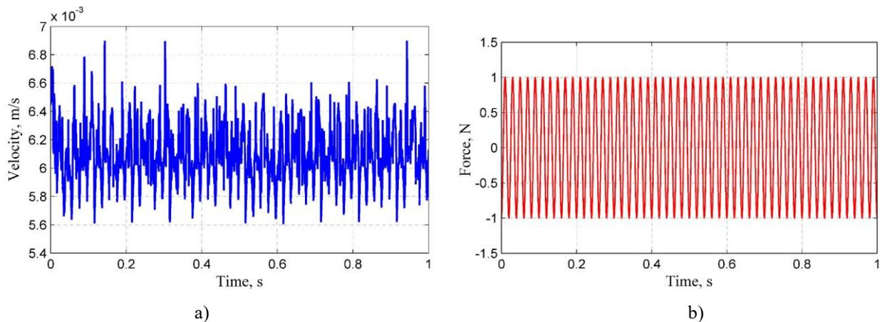
Fig. 5. The example of measuring data from test: a) scanning signal by PSV-400 scanning head on tire surface; b) impulse generated by piezoelectric element on the inner surface of tire.
