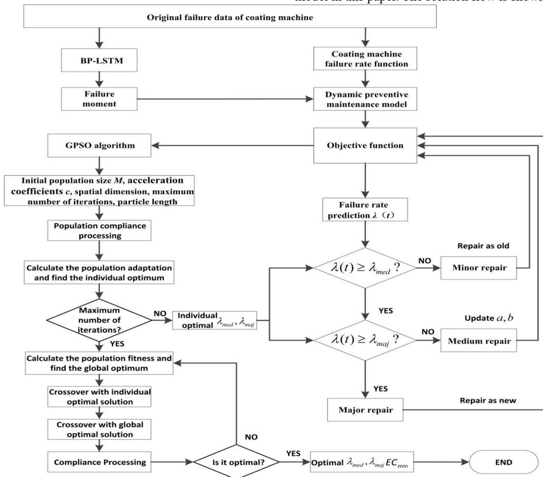
Fig. 7. Flow chart of dynamic preventive maintenance model solving based on GPSO algorithm.
