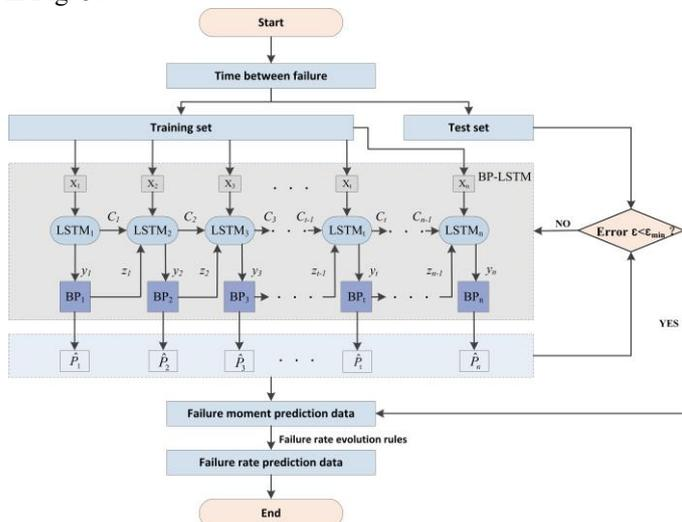
Fig. 5 Failure rate prediction framework based on BP-LSTM.
