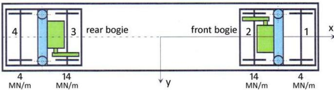
Fig. 18. Visualization of traction motor alignment for the subway car model with unsymmetric primary suspension stiffness arrangement 4-14-14-4.
