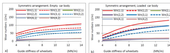
Fig. 4. Wear numbers for wheels of metro wagon models with symmetric arrangement on the full arc of curved track with a radius of 300 m: a) empty car body, b) loaded car body.
