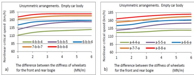
Fig. 6. Changes of nonlinear critical speed of metro wagon model with empty car body in function of difference between the guide stiffnesses of wheelsets for the front and rear bogie with unsymmetric arrangements; a) first scenario, b) second scenario.
