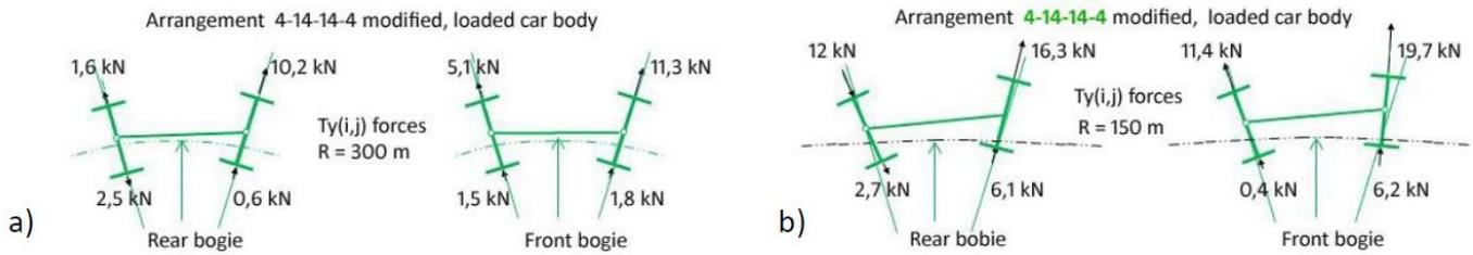
Fig. 17. Values of lateral tangential forces  $T_y(i, j)$  acting on the wheels of wheelsets of the front and rear bogies on curved track for modified unsymmetric arrangement 4-14-14-14: a) curved track with radius of 300 m, b) curved track with radius of 150 m.
