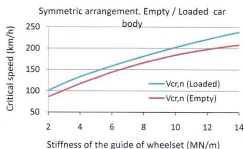
Fig. 3. Nonlinear critical speeds  $v_{cr,n}(E)$  and  $v_{cr,n}(L)$  in function of the guide stiffness of wheelsets in bogie frame of the metro wagon model with empty and loaded car body for symmetric arrangement.
