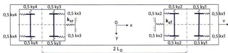
Fig. 2. Plan view of the phenomenological model of the primary suspension and of the traction rod.
