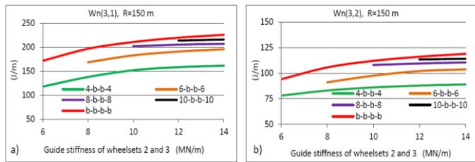
Fig. 11. Comparison of wear number values for the wheels of leading wheelset of rear bogie on curved track with the radius of 300 m for symmetric **b-b-b-b** and unsymmetric **4-b-b-4** arrangements: a) left wheel, b) right wheel.
