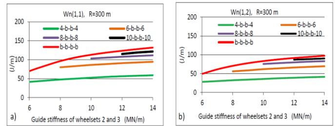
Fig. 8. Comparison of wear number values for the wheels of leading wheelset of front bogie on curved track with the radius of 300 m for symmetric **b-b-b-b** and unsymmetric **4-b-b-4** arrangements; a) left wheel, b) right wheel.
