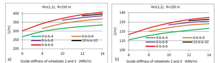
Fig. 10. Comparison of wear number values for the wheels of leading wheelset of front bogie on curved track with the radius of 150 m for symmetric **b-b-b-b** and unsymmetric **4-b-b-4** arrangements: a) left wheel, b) right wheel.
