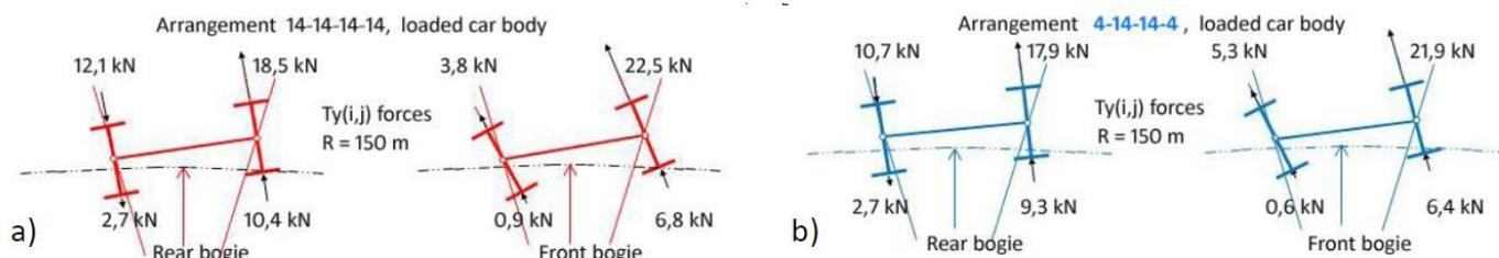
Fig. 16. Values of lateral tangential forces  $T_y(i, j)$  acting on the wheels of wheelsets of the front and rear bogies on the curved track with radius of 150 m: a) symmetric arrangement **14-14-14-14**, b) unsymmetric arrangement **4-14-14-14**.
