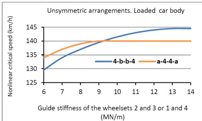
Fig. 7. Comparison of nonlinear critical speed values of metro wagon model with loaded car body in function of guide stiffness of wheelsets for **4-b-b-4** and **a-4-4-a** arrangements.
