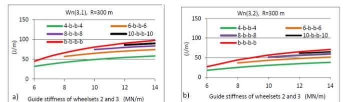
Fig. 9. Comparison of wear number values for the wheels of leading wheelset of rear bogie on curved track with the radius of 300 m for symmetric **b-b-b-b** and unsymmetric **4-b-b-4** arrangements: a) left wheel, b) right wheel.
