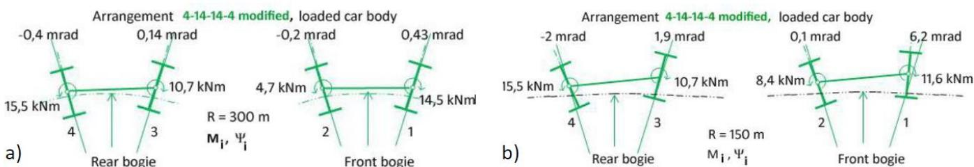
Fig. 14. Alignments of leading and trailing wheelsets of the front and rear bogies on curved track for modified unsymmetric arrangement **4-14-14-14**: a) curved track with radius of 300 m, b) curved track with radius of 150 m.
