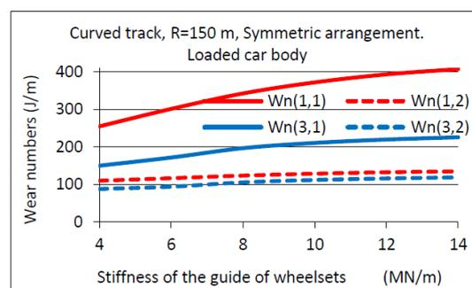
Fig. 5. Wear number values for the wheels of leading wheelsets of metro wagon model with loaded car body on curved track with the radius of 150 m.
