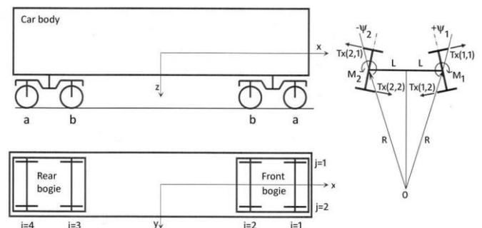
Fig. 1. Elements of the reference metro wagon model and interpretation of signs of angles of attack of wheelsets and moments  $M_i$  generated by the longitudinal tangential forces  $Tx(i, j)$  on curved track in case of the front bogie.
