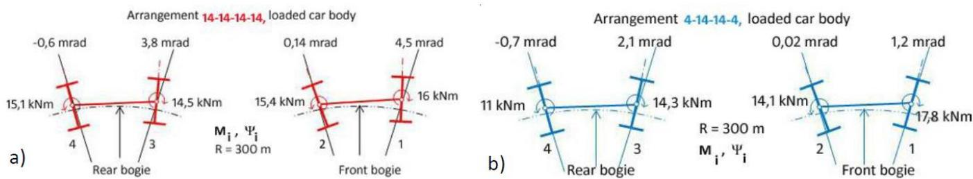
Fig. 12. Alignments of leading and trailing wheelsets of the front and rear bogies on curved track with radius of 300 m: a) symmetric arrangement **14-14-14-14**, b) unsymmetric arrangement **4-14-14-14**.
