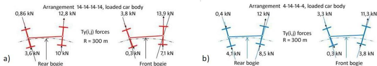
Fig. 15. Values of lateral tangential forces  $T_y(i, j)$  acting on the wheels of wheelsets of the front and rear bogies on the curved track with radius of 300 m: a) symmetric arrangement **14-14-14-14**, b) unsymmetric arrangement **4-14-14-14**.
