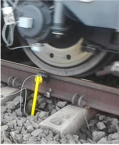
Fig. 10. Views of analysed track sections a) tested weld, b) rail deflection measurement without weld.
