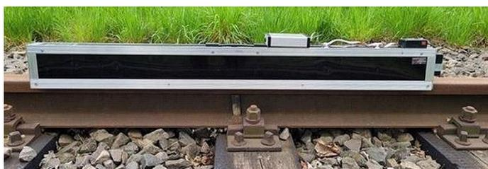
Fig. 2. PRS02W laser profilometer used for tests.
