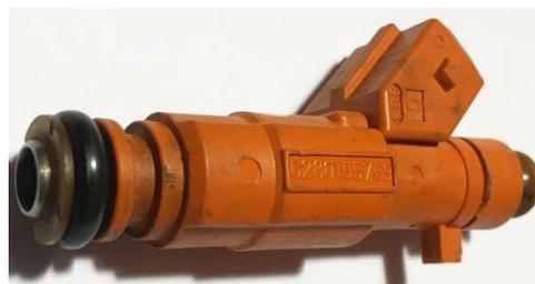
Fig. 1. Electromagnetic fuel injector.
