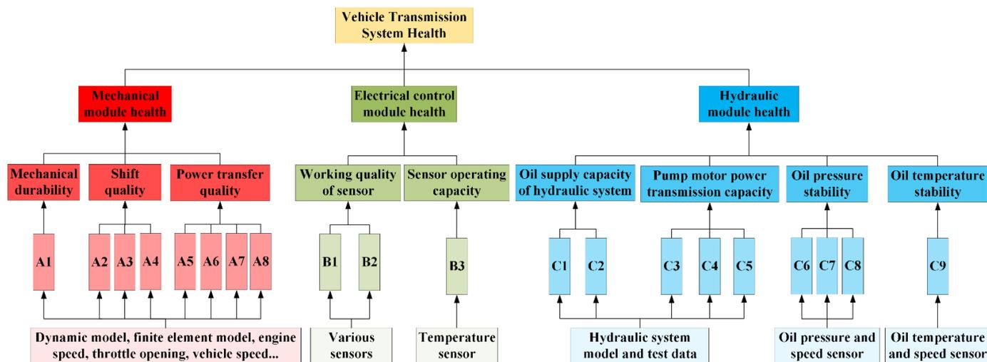
Fig.1. Comprehensive transmission device performance parameter level.
