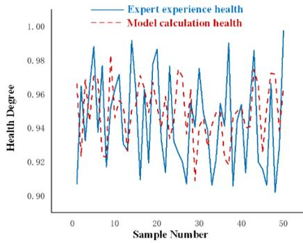
(a) Single mechanical module level health degree.
