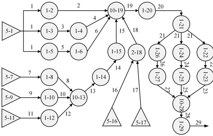
Fig. 2. GO diagram of PMSM drive system
