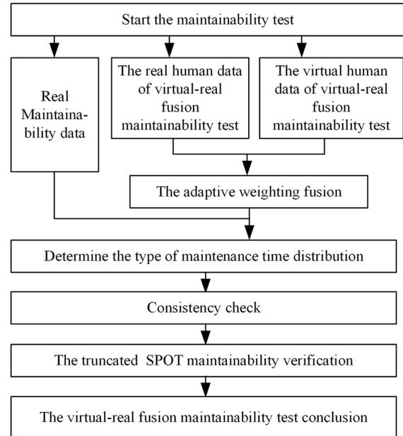
Fig. 4. Virtual–real fusion maintainability evaluation test method
