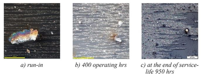
Fig. 10. Spectro T<sup>2</sup>FM ferrograph images showing metal particles in engine oil over the lifetime of an internal combustion engine
