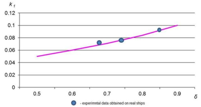
Fig. 7. Dependence of coefficient  $k_1$  on the ship's block coefficient
