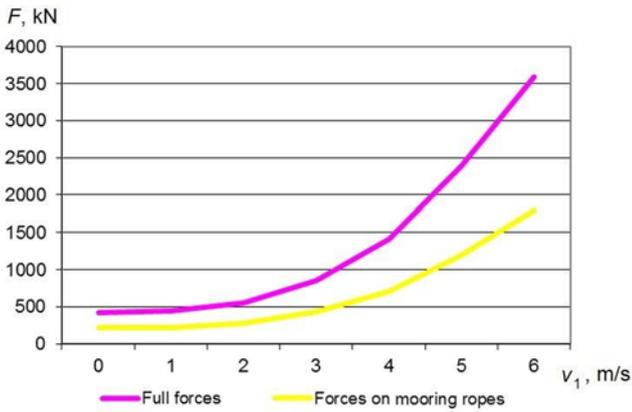
Fig. 15. Dependence of total forces (F) acting on moored vessel and forces acting on mooring ropes on speed (v1) under the set conditions
