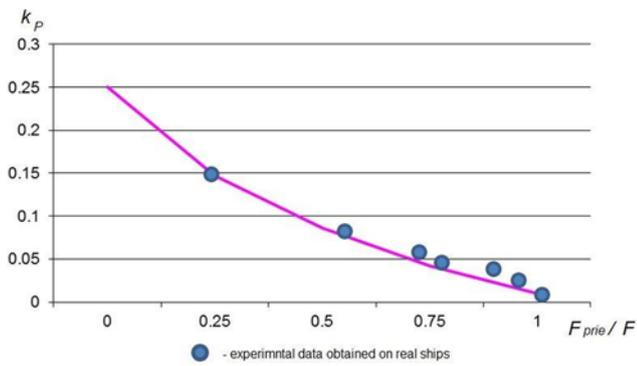
Fig. 10. Dependence of mooring rope pretension coefficient  $k_P$  on the mooring rope pretension and total external forces acting on moored ship  $F_{prie} / F$
