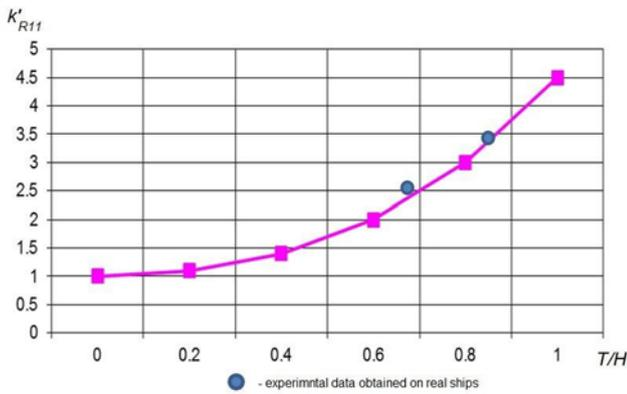
Fig. 9. Dependence of ship's resistance coefficient  $k'_{R11}$  on ship's draft and depth  $T/H$
