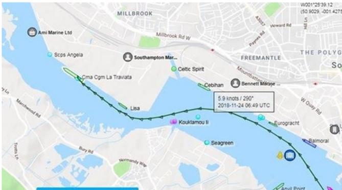
Fig. 3. Container vessel "CMA CGM La Traviata" ( $L = 334$  m,  $B = 43$  m,  $T = 13$  m) passing through narrow channel close to the moored ships in Southampton port (UK) [1]
