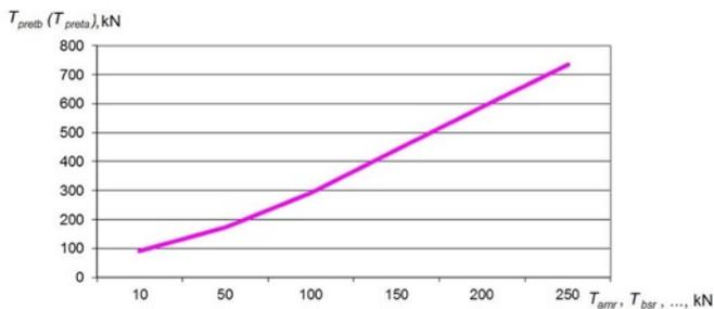
Fig. 16. Dependence of total mooring rope pretension forces in one direction (bow or astern) on each mooring rope pretention
