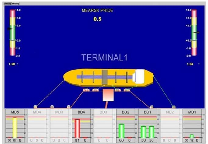
Fig. 11. Laser "Dockmaster 3" measuring system, implemented on quay walls No. 1 and No. 2 in Klaipeda port ring rope pretension and total external forces acting on moored ship  $F_{prie} / F$
