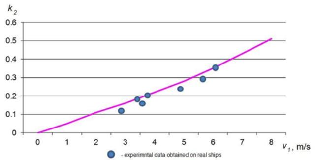
Fig. 8. Dependence of coefficient  $k_2$  on the passing ship's speed
