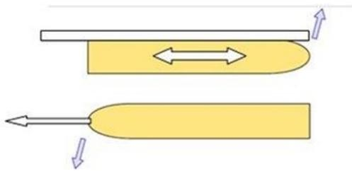
Fig. 6. The influence of passing ship on a moored vessel, where: purple arrow – forces that turn the ship, white arrow – ship's moving direction
