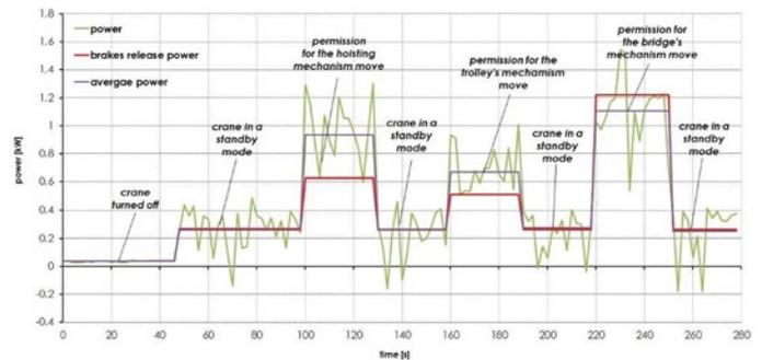
Fig. 5.1. Power demand of the overhead crane.
