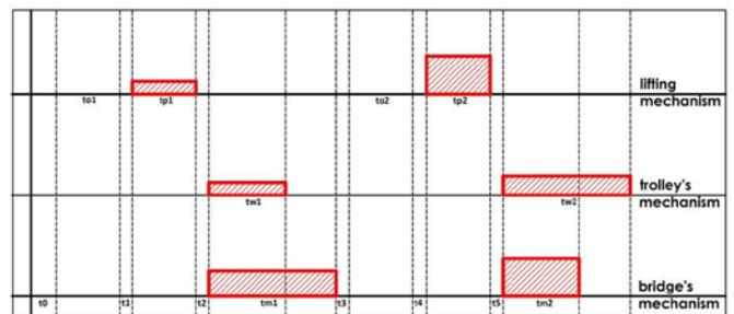
Fig. 5.6. Crane's duty cycle without possibility of restoring the energy
