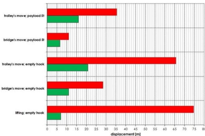
Fig. 5.8. Potential savings after lowering the 5 tons payload from the 5 meters height.
