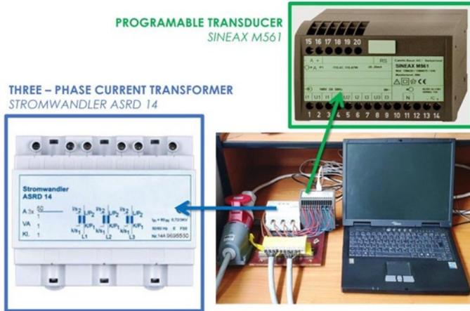
Fig. 3.3. Intermediary measuring system plugged between the crane's drive control and the power grid
