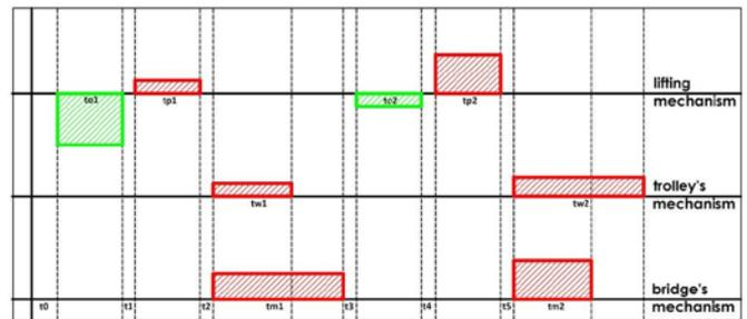
Fig. 5.5. Crane's duty cycle with possibility of restoring the energy
