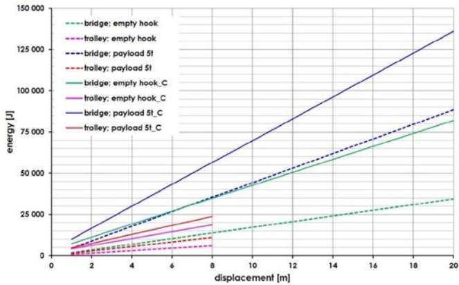
Fig. 5.2. Energy consumption of the overhead crane for the bridge and trolley mechanisms related to the travelled distance for different loading conditions
