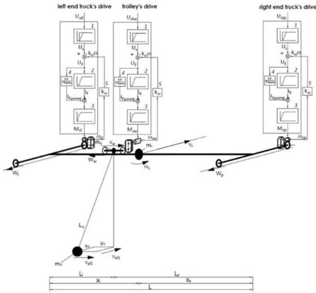
Fig. 3.2. The model of overhead crane drive system with a suspended payload
