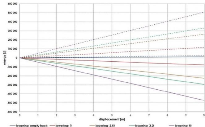
Fig. 5.3. Energy consumption of winch mechanism in relation to the travelled distance (lifting and lowering) for different loading conditions.
