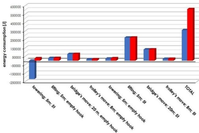
Fig. 5.7. Comparison of two types of duty cycle both with the energy saving system (blue) and without (red)
