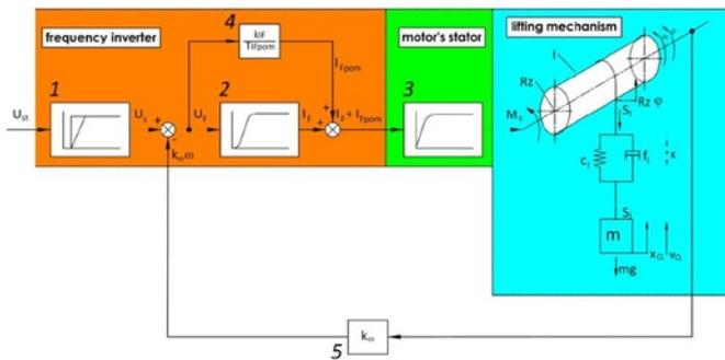
Figure 3.1. The model of the hoist and the inverter – motor's stator [13]
