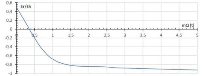
Fig. 5.4. The possibility of energy recuperation during lowering with respect to energy consumption during hoisting.
