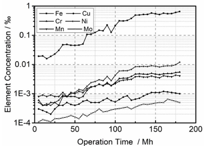
Fig. 4. Spectral oil data for one PSST system
