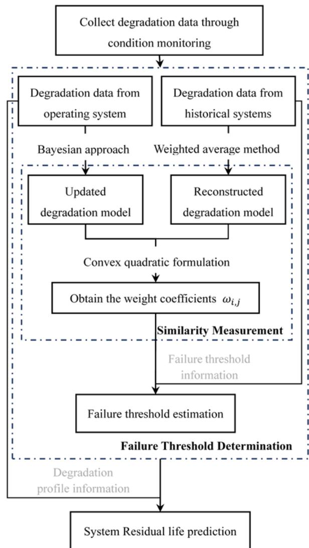
Fig. 1. Failure threshold determination framework for RL prediction
