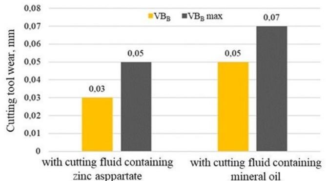
Fig. 7. Wear indices of cutting tools made of HS6-5-2C steel after turning with cutting fluids
