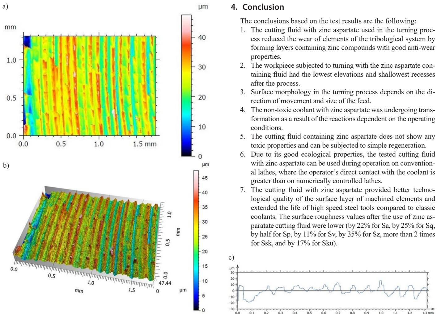
Fig. 10. Geometric structure of the workpiece edge after turning with a cutting fluid containing zinc aspartate: a) contour map, b) isometric image, c) primary profile
