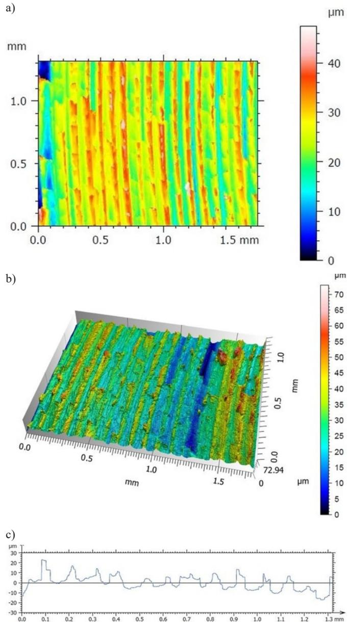
Fig. 9. Geometric structure of the workpiece edge after turning with the cutting fluid containing mineral oil: a) contour map, b) isometric image, c) primary profile
