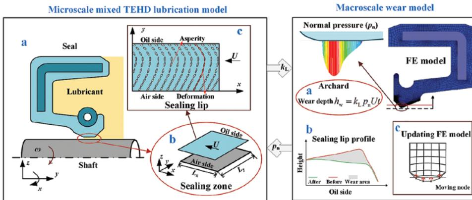
Fig. 1. Schematic diagram of wear degradation model
