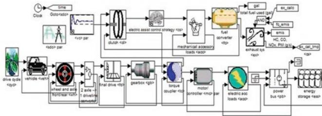
Fig. 4. Model of parallel hybrid vehicle in ADVISOR
