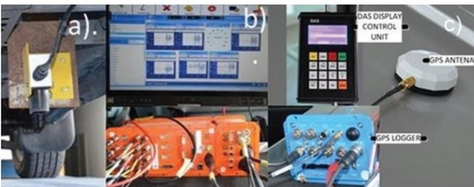
Fig. 2. Measurement equipment used to conduct the tests in real-world conditions
