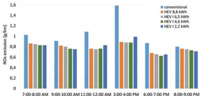
Fig. 10. NO<sub>x</sub> emission during trips at specific times of day
