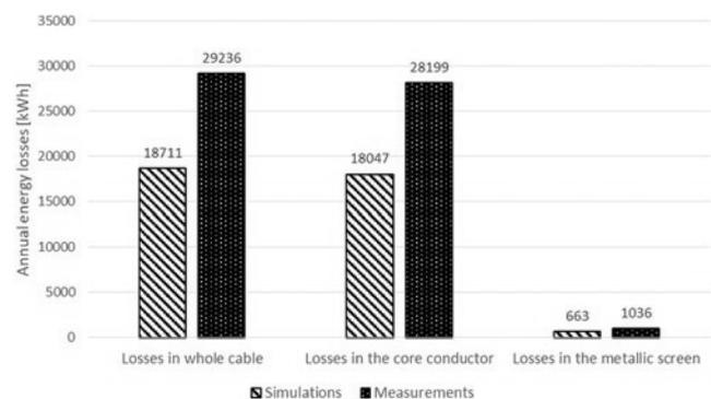
Fig. 7. Comparison of summed cable screen annual losses in investigated cable sections obtained from simulation and measurement results
