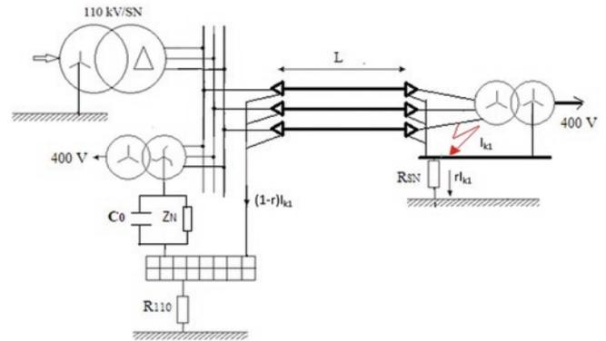
Fig. 11. Phase to earth current flow during the earth fault at MV/LV substation, including cable screens of the cable, as well as resistance of earthing systems of both substations;  $Z_N$  – impedance of MV neutral point earthing (resistor or Petersen's coil),  $C_0$  – earth fault network capacitance,  $I_{k1}$  – earth fault current,  $R_{110}$  – earthing resistance of the HV substation,  $R_{MV}$  – earthing resistance of the MV substation,  $L$  – length of the considered cable line [km]
