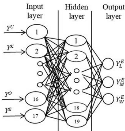
Fig. 2. Structure of the created MLP 17-19-3 network
