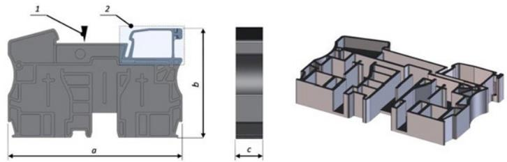
Fig. 2. The model of the electrical connector fitted with flexible joint parts: a = 80,2 mm, b = 50,6 mm, c = 12,2 mm, 1 – injection point, 2 – the forming area of the flexible installation foot qualified for selective induction heating
