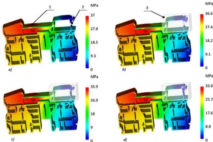
Fig. 3. Simulation tests of filling the mold cavity for electrical connector housing, a) conventional process with constant mold temperature, b) temperature of induction heated area is 130°C, c) temperature of induction heated area is 150°C, d) temperature of induction heated area is 170°C, 1 – injection point, 2 – the place of joining of flowing plastic streams, 3 – the mold area heated by induction heating
