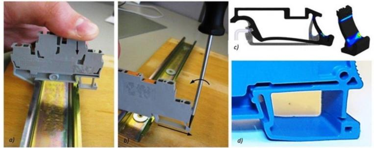
Fig. 1. Example of an electrical connector fitted with a flexible clip: a) assembly of connector on the rail, b) disassembly of the product using a screwdriver, c) stress concentration in the flexible clip during disassembly process, d) the problem of cracking of the installation foot during deformation of the clip
