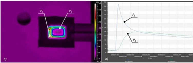
Fig. 6. Examples of results displayed in the FLIR Research MAX program: a) thermogram, b) graph,  $P_1$  – placed straight on the heated wall and  $P_2$  – placed 1 mm into the material from the heated surface
