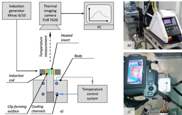
Fig. 5. Experimental tests of induction heating process carried out on the insert which forms the molded part's clip: a) a diagram b), c) the test stand
