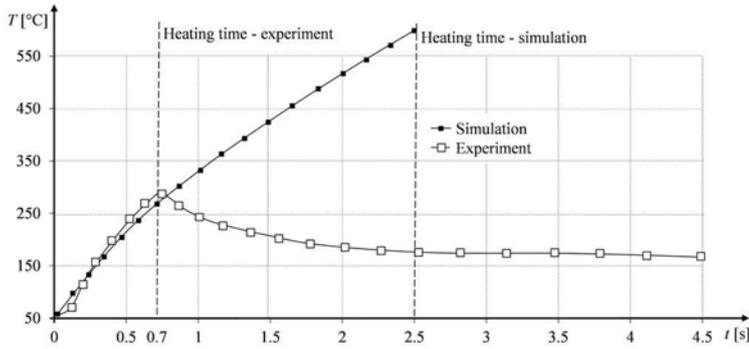
Fig. 7. Comparison waveforms of the heating process for simulation and experimental studies while keeping 1 mm gap between induction coil and the heating surface
