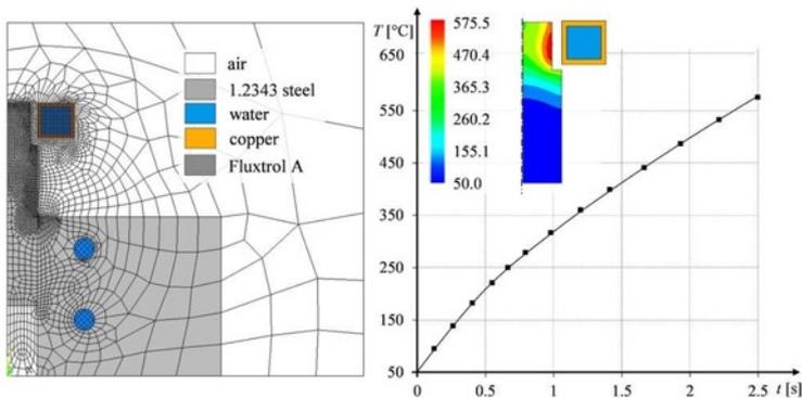
Fig. 4. Simulation tests of induction heating process carried out on the insert which forms the molded part's clip: a) a diagram with a preset discretisation in a Quick-Field program b) obtained results
