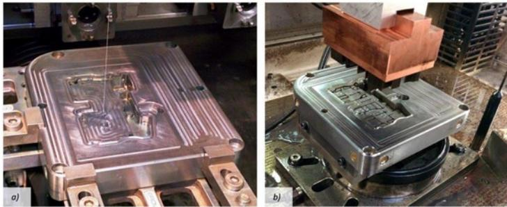
Fig. 8. Preparation of the mold cavity: a) making of ejector holes in wire electrical discharge machining technology, b) making of shapes which form a ribbing of the molded part
