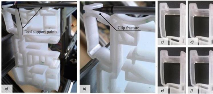
Fig. 9. Samples made for assembly tests: a) disassembly process of the housing from the rail, b) the phenomenon of cracking of the flexible clip during the disassembly of the housing, c) view of the clip made by using the conventional method, d) view of the clip made by using the induction heating,  $T = 130^{\circ}\text{C}$ , e)  $T = 150^{\circ}\text{C}$ , f)  $T = 170^{\circ}\text{C}$
