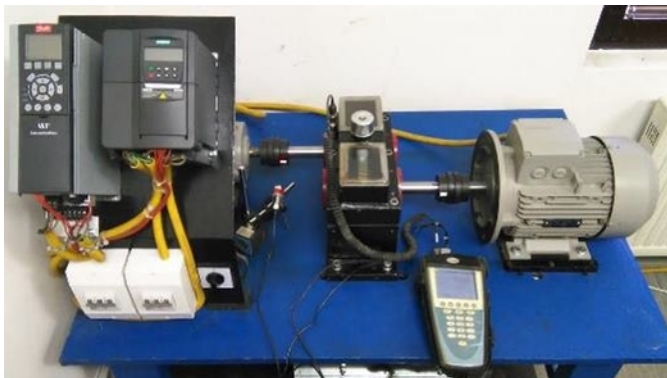
Fig. 3. Gearbox test bench
