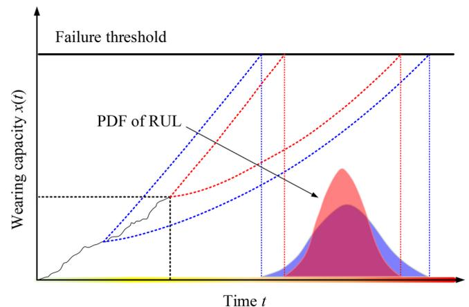
Fig. 1. Diagram of degradation process
