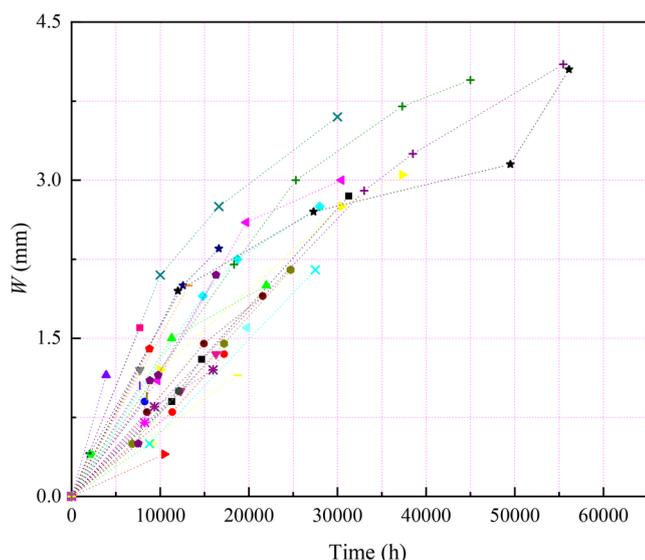
Fig. 3. Wear path of the cylinder liners [13]
