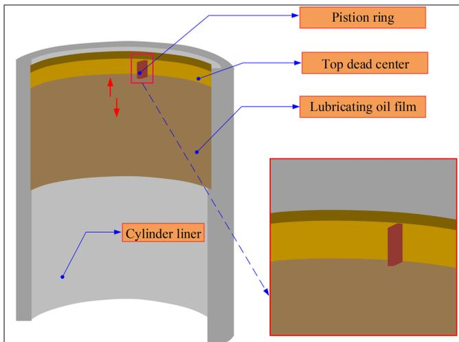
Fig. 2. The wear diagram of the cylinder liner
