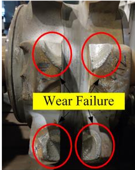
Fig. 2. Component failure on shearer
