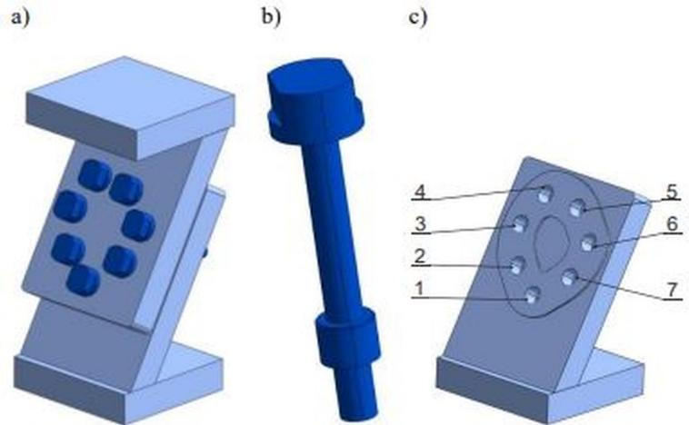
Fig. 1. Model of the connection: (a) model 3D, (b) model 3D of the single fastener, (c) outline of the surface at the contact of the joined plates and assumed numbering of the bolts
