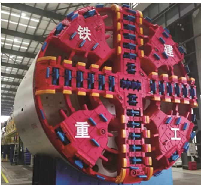
Fig. 2. The selected EPBM used in this project
