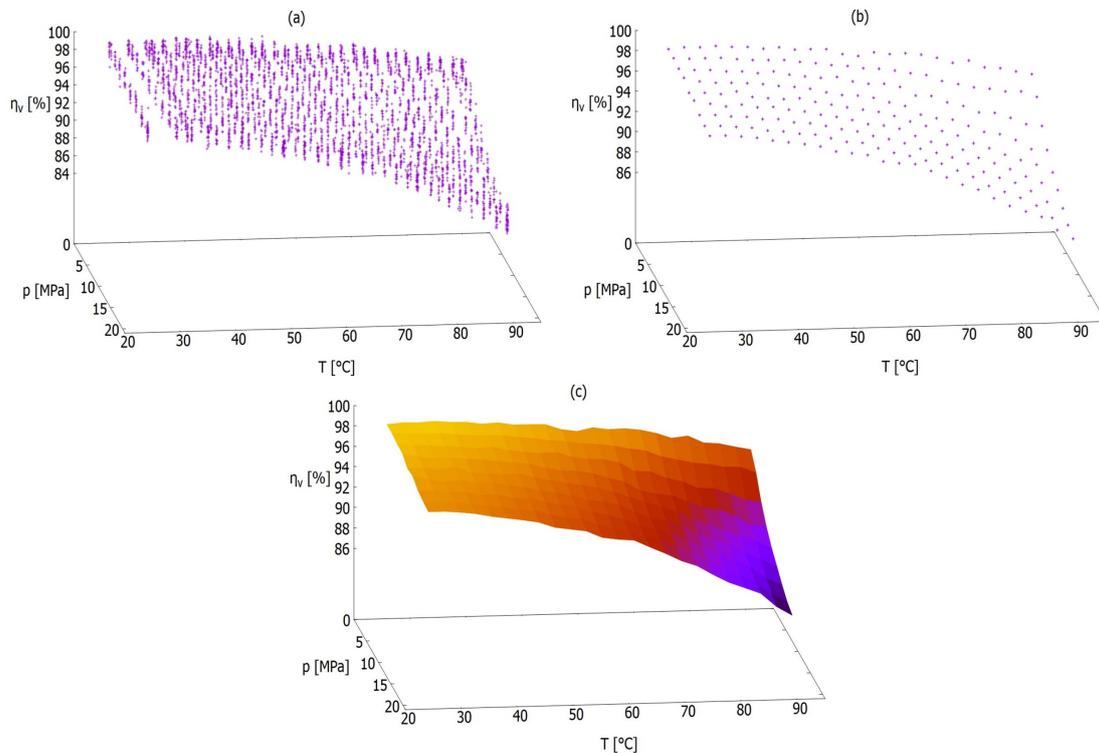
Fig. 4. Sample map of measurement points from the Gnuplot software: (a) after noise reduction, (b) after dgrid3d function, (c) after data processing
