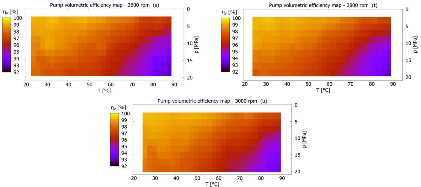
Fig. 5. Volumetric efficiency maps for different speeds
