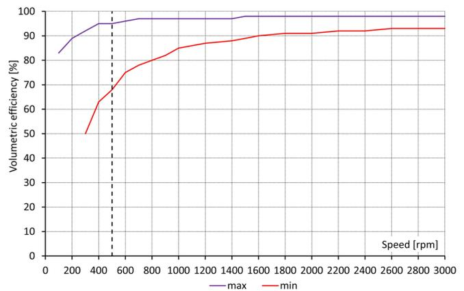
Fig. 6. Volumetric efficiency range for 17 MPa operating pressure
