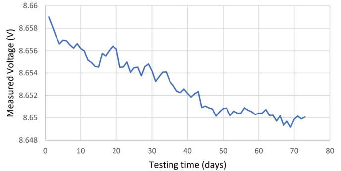
Fig. 9. Diagrams of the voltages measured from LED nr. 8 from the beginning of the test to the first voltage jump
