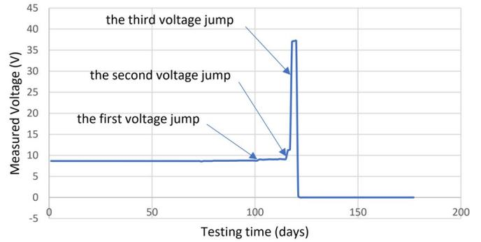
Fig. 8. Diagrams of the measured voltages of LED nr. 8
