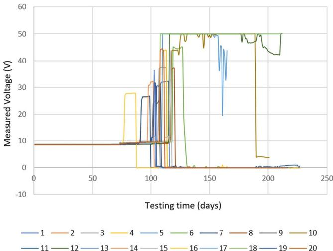
Fig. 7. The graphs of the measured voltages of the LEDs from the accelerated test
