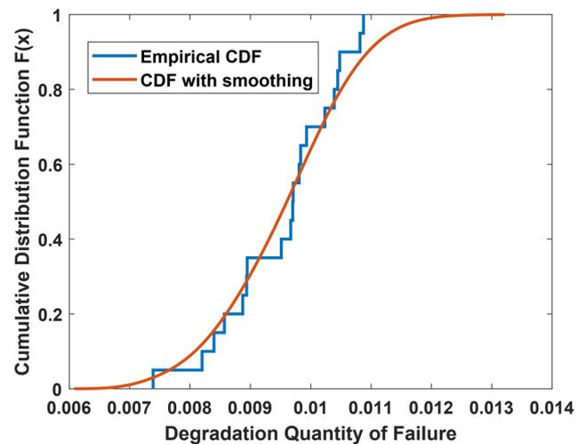
Fig. 11. The graph of CDF of the data using nonparametric methods
