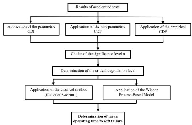
Fig. 1. The main steps of the mean time to soft failure determination process
