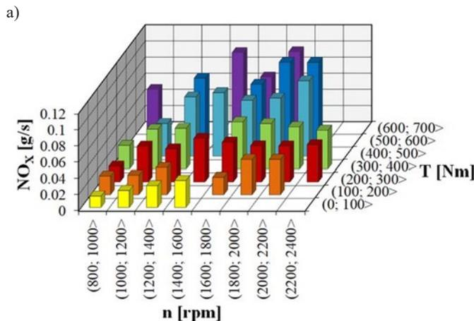
Fig. 9. Characteristics of a) second NO<sub>x</sub> emission rate b) NO<sub>x</sub> toxicity in the torque ranges of the engine speed
