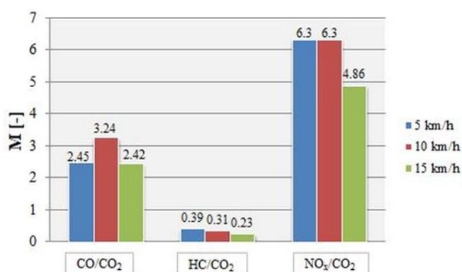
Fig. 10. Comparison of M emission indicators for CO, HC and NO<sub>x</sub> obtained during the three test drives
