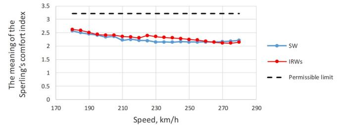
Fig. 10. The value of the Sperling's comfort index in the vertical direction in tangent track
