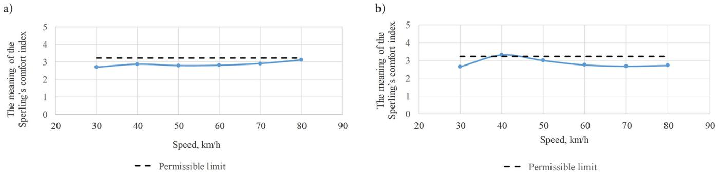
Fig. 16. Experimental Sperling's comfort index values at different running speeds: a) in vertical direction; b) in lateral direction
