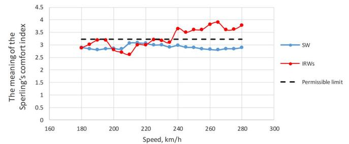
Fig. 11. The value of the Sperling's comfort index in the lateral direction in tangent track
