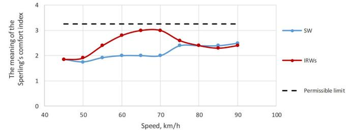
Fig. 4. Sperling's comfort index values in the lateral direction in 200 m radius curve
