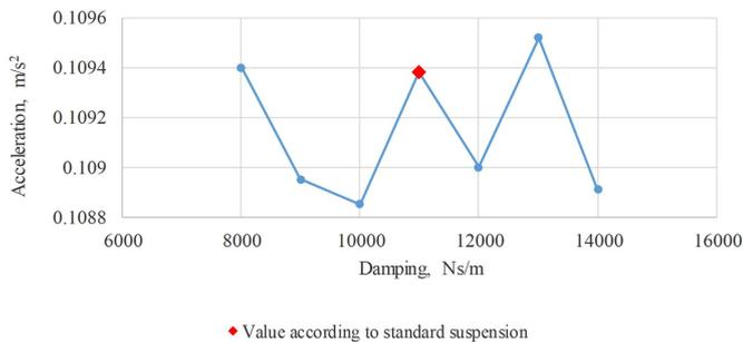
Fig. 9. Dependence of mean square body accelerations on secondary suspension damping parameters
