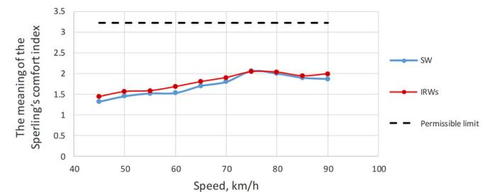
Fig. 12. The value of the Sperling's comfort index in the vertical direction in a 200 m radius curve
