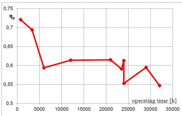
Fig. 9. Dependence of average pump efficiency on time
