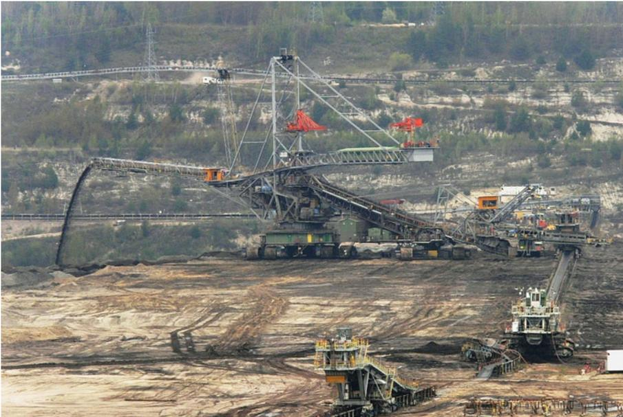
Fig. 1. Spreader A<sub>2</sub>RsB 15400 – typical example of opencast mining machinery (photo. P. Grabowski)
