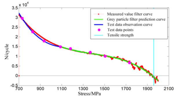
Fig. 19. P-S-N curve modified by grey particle filter
