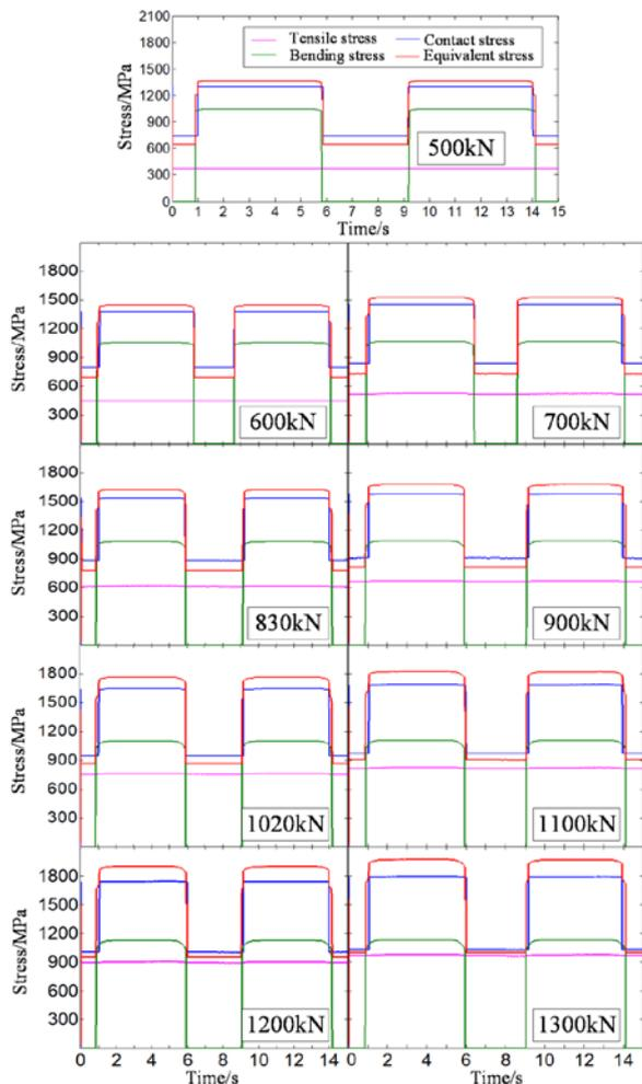
Fig. 8. Stress-time history curve under tension conditions
