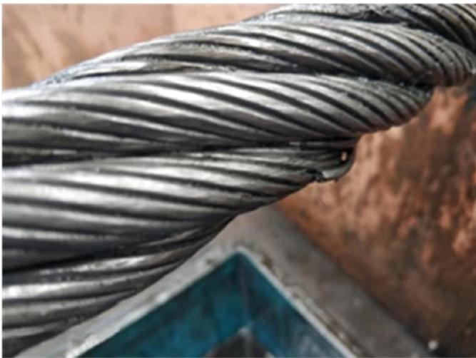
Fig. 3. Actual fracturing part of wire rope
