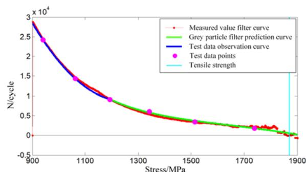
Fig. 21. P-S-N curve of the second set after grey particle filtering
