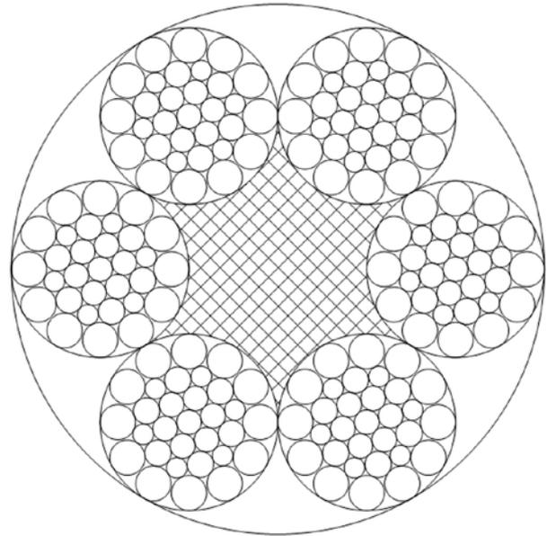
(b) Wire rope section view
