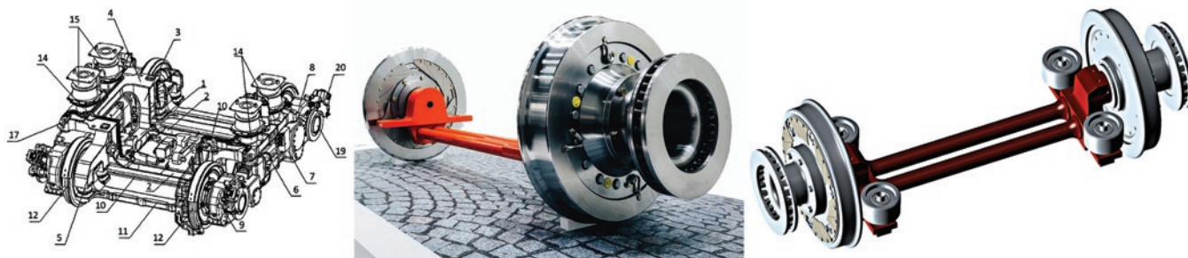
Fig. 2. Low-floor tram vehicle motor bogie with cranked axles [50,16]
