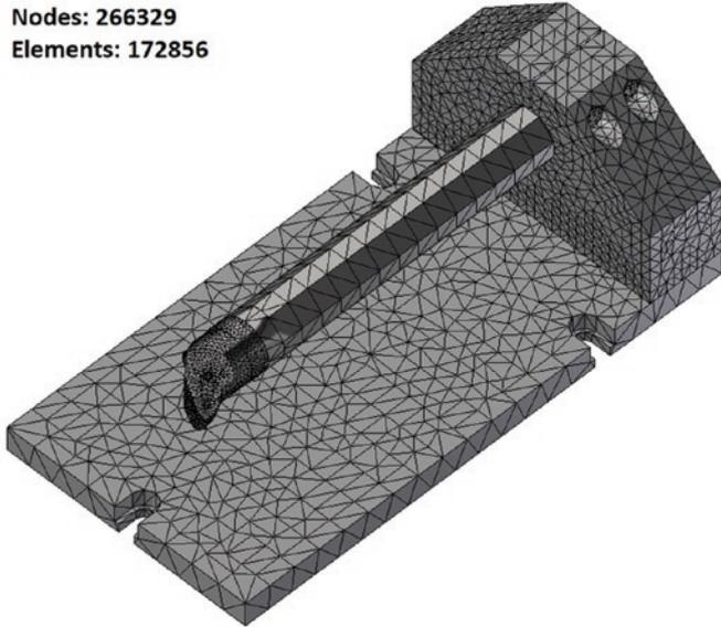
Fig. 2. Finite element mesh view
