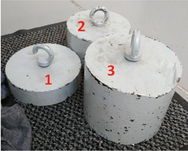
Fig. 9. View of the prepared weights: 1 – 10 kg, 2 – 20 kg, 3 – 30 kg
