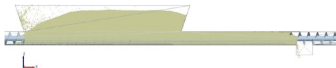
Fig. 11. Simulated transportation of the material by a screw conveyor
