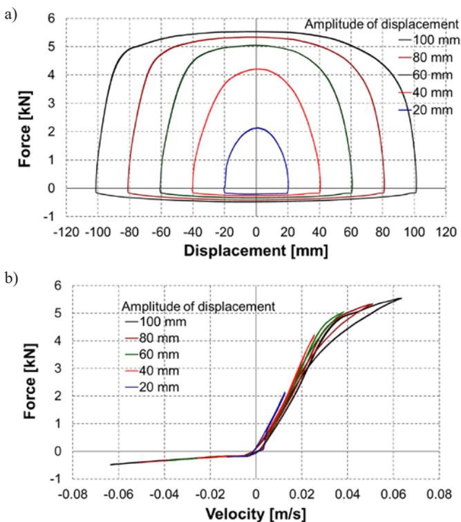
Fig. 2. Force-displacement and force-velocity characteristics of the shock absorber
