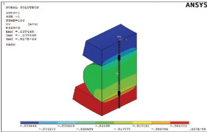
Fig. 18. Displacement of radial cylindrical roller bearing elements
