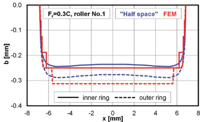
Fig. 16. Contact areas of a roller with raceways
