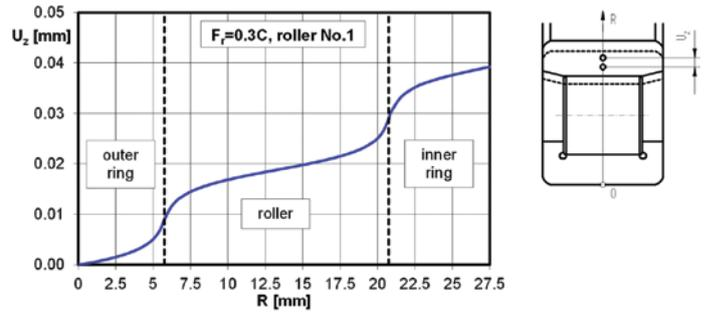
Fig. 19. Local displacement  $U_z$  inside the bearing elements
