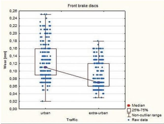
Fig. 3. Wear of the front brake discs component depending on the type of traffic
