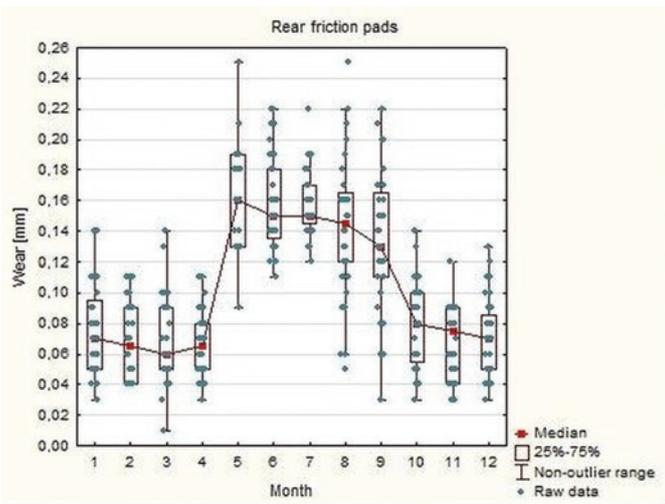
Fig. 11. Wear of the rear brake discs component depending on the month
