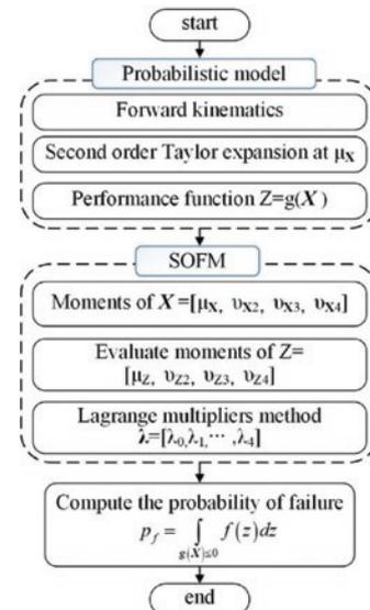
Fig. 3. Procedure of reliability analysis with SOFM
