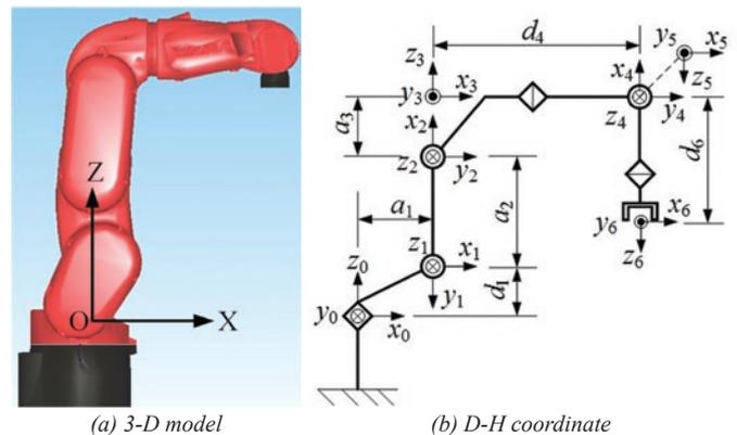
Fig. 1. A schematic diagram of a serial manipulator
