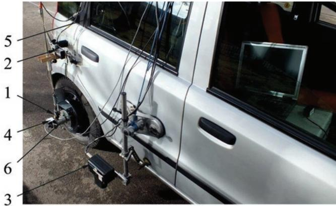
Fig. 6. Test object with mounted measuring apparatus
