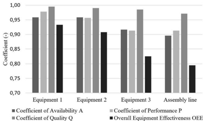
Fig. 4. Results of OEE calculation for serial system
