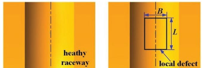
Fig. 6. Models of healthy outer raceway and outer raceway with local defect
