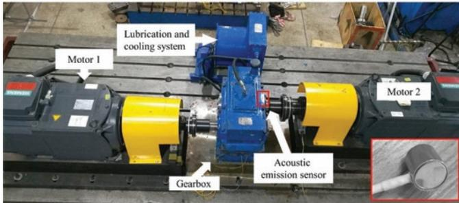
Fig. 4. Schematic of the gearbox test rig
