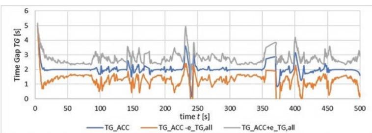
Fig. 16. Time Gap for a car with ACC taking into account  $e_{TG, all}$  parameter (in case of constant vel of tracked car) in task 2
