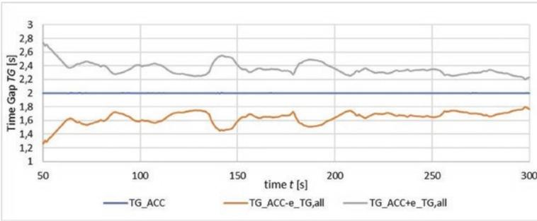
Fig. 9. Time Gap for a car with ACC taking into account  $e_{TG, all}$  parameter (in case of constant vel of the tracked car) in task 1
