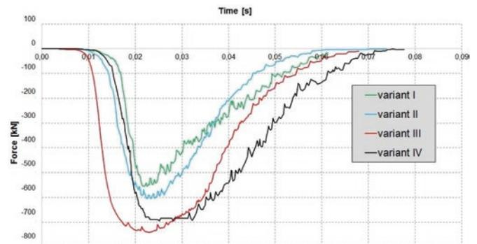
Fig. 10. Comparison of trimming forces for all variants
