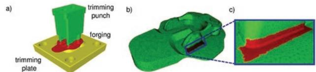
Fig. 7. View of: a) a diagram of the trimming process, b) a meshed up forging before trimming for the whole forging, c) densification of the web on the trimming line with the use of “meshboxes”
