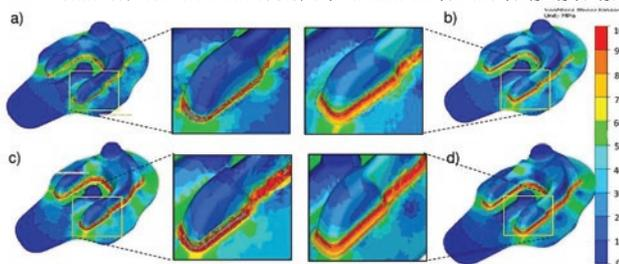
used forging tools with flash at the level above 2.2 mm and worn-out trimmin tools, d) variant IV - for the forgings made of new tools for forging with flash 2 mm and worn-out trimming tools
