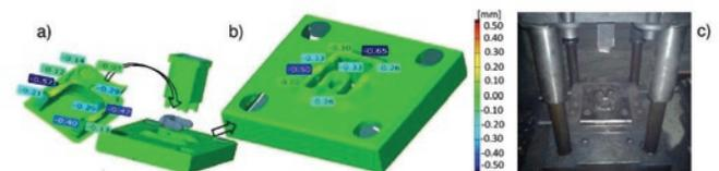
Fig. 8. Measurement-scanning results for trimming tools: a) a punch, b) a die (cutting plane), c) view of trimming device
