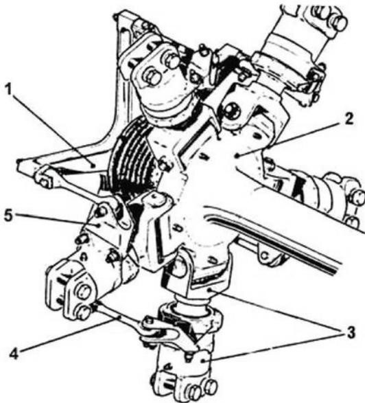
Fig. 1. Rotor hub assembly [4]
