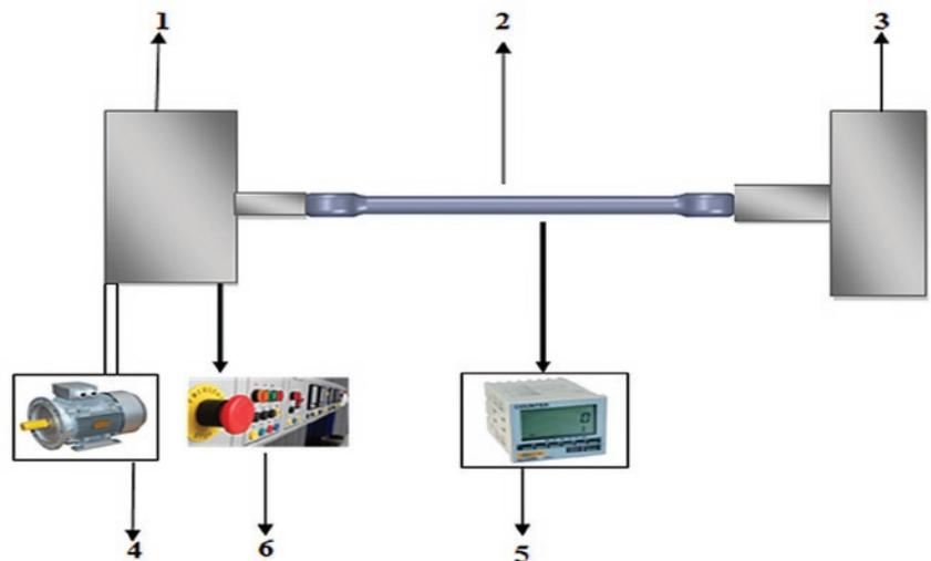
Fig. 3. Testing bench for the rotor pitch links
