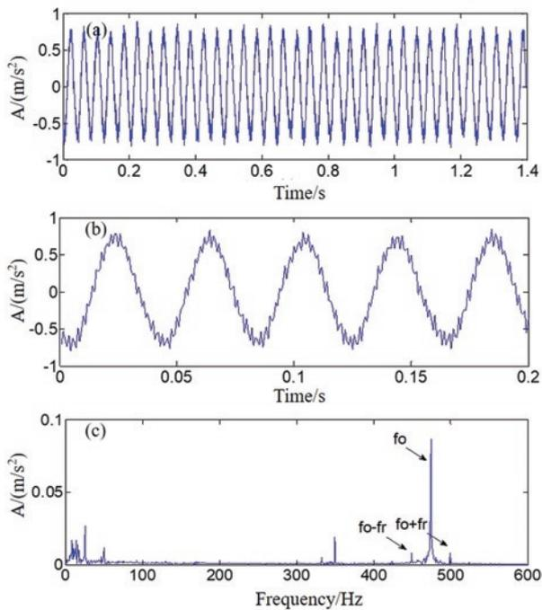
Fig. 11. The analysis of denoising results of NLM in case study 2: (a) denoising signal, (b) local amplification of the denoising signal and (c) envelope spectrum of denoising signal
